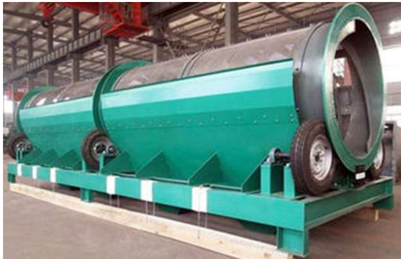
Criba minera. Fuente: http://spanish.industrialcrushermachine.com/sale-9554074-rotary-trommel-screen-mining-vibrating-screen-fully-enclosed-structure-5-35-mm-aper-ture.html
